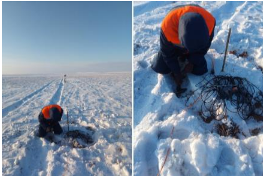
Figure 3.3.2.1 – Installation process of geophones in SP
