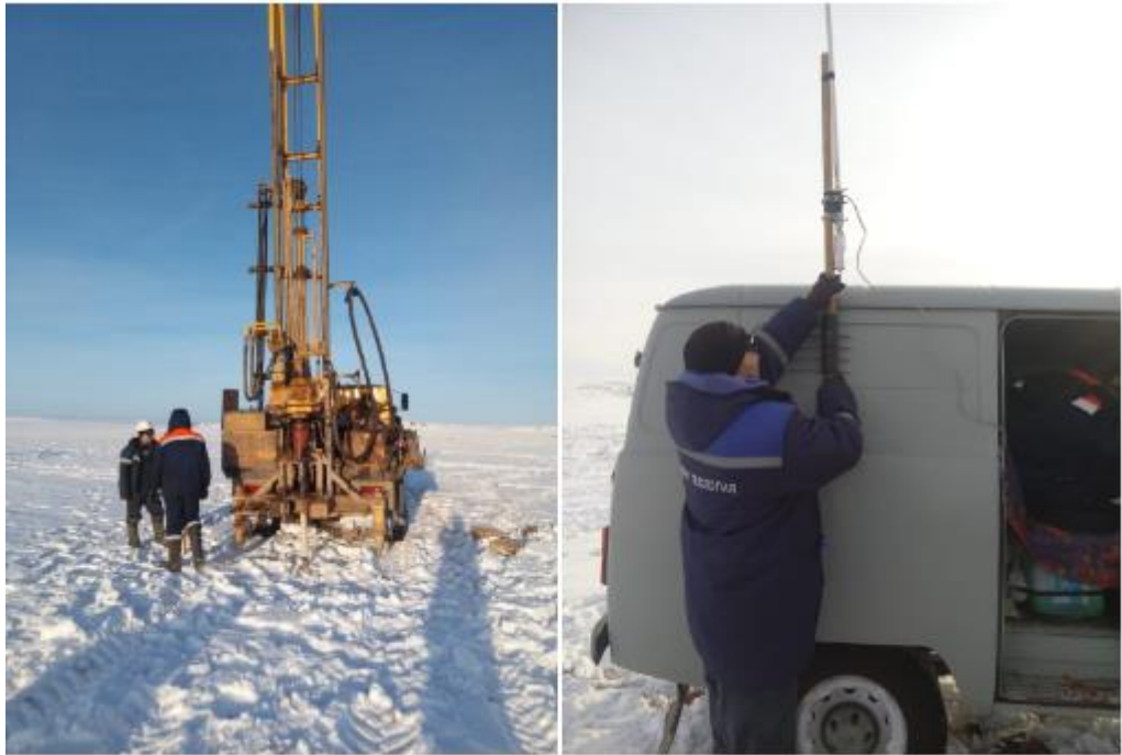
Figure 3.3.5.1 – URB-2A2 Drilling rig and uphole survey station
